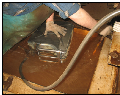
Hermetism test – 0.3 bar
